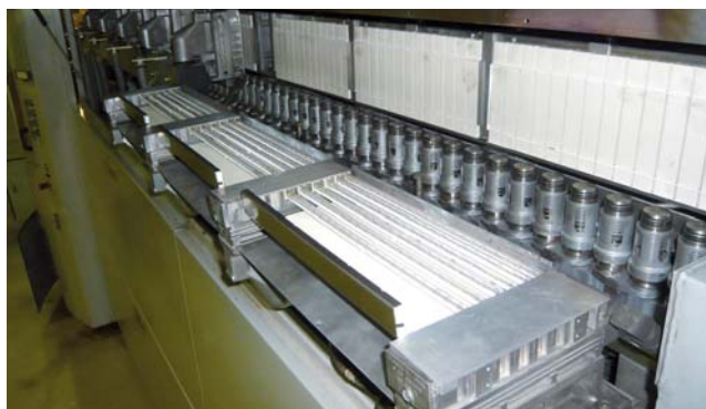
Preform oven with heat shields and ceramic reflectors
