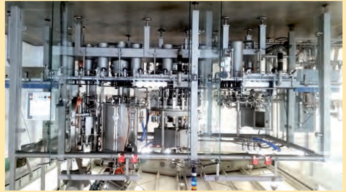
“All-in-One” rinser/ filler/capper block for glass and PET bottles as well as cans
