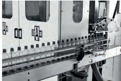
Figure 3.4 Stand-up conveyors are most commonly used at the end of linear machines. Photo courtesy of W. Amsler Equipment Inc.
