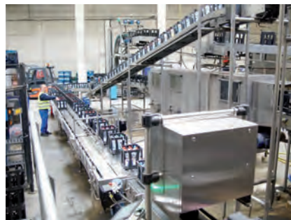
Removed cases with errors are corrected manually and placed back into the production flow.
