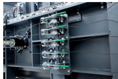
New bale measuring system for exact determination of the bale length
