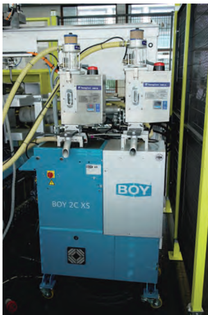
The dehumidification unit – in this case the Card G – is mounted on the injection moulding machine outside the feeder and permanently supplies the small material container with dried resin. (Photos: Dr. Boy GmbH & Co. KG, FarragTech GmbH)
