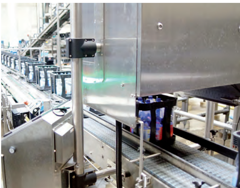
Up to 7,000 cases per hour are checked against numerous criteria by a dual lighting module and ultrasound sensors.
