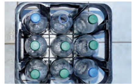
Tricky for the cameras and sensors to recognise are the “correct” PETCycle bottles with eight or ten-sided neck rings.
