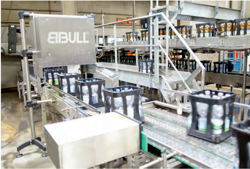
Cases with recognised errors are carefully transferred by the pneumatic “Sinus Sorter” to a parallel conveyor and transported for manual checking.
