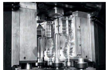
Figure 3.2 Most preforms are blown upside down on this type of blow-moulding machine. Photo courtesy of Chumpower Machinery Corp.
