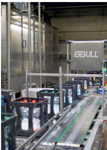
The empties cases are brought at a set distance before the measuring bridge of the "BBull 500 Compact LG", checked and errors are sorted out.
