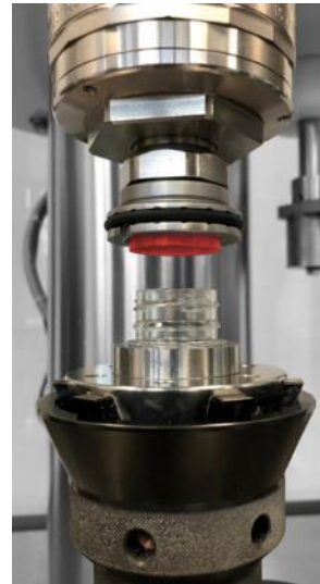
Closure in chuck neck 1mm off-center
