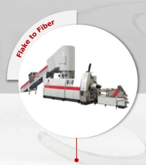
Various solutions for PES recycling including hybrid lines flake/fiber, ultra-fine filtration with sleeve/candle filter and IV increase in melt phase or solid state
