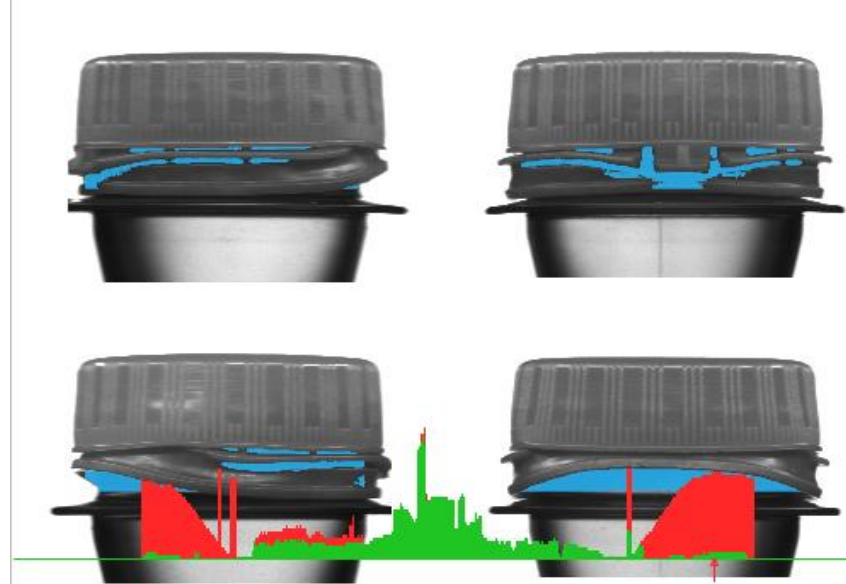
Defects found exceeding histogram
