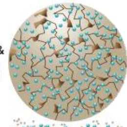
Desiccant Deterioration on 18 to 24 months
